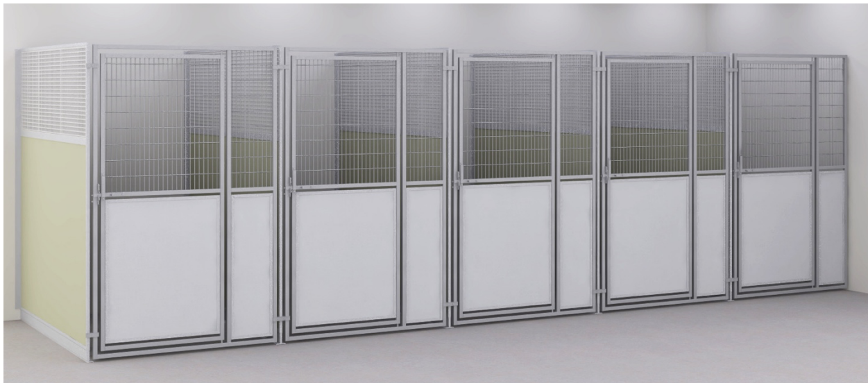
2: Kennel rendering shown here is a standard depth of 6'. Kennels by Midmark to be installed at SHS are custom 12' deep. The kennel design includes frosted fronts on the bottom half and will include a wire grid over the kennel tops.
